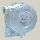
EDA-22 systems monitor air flow, dirty filters, flue draught, frost on coils & level. For positive, negative, vacuum & differential pressure. Suitable for non-corrosive, non-combustible air/gases.
